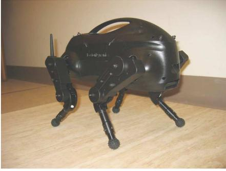
Fig. 4. The LittleDog robot, designed and built by Boston Dynamics, Inc.
